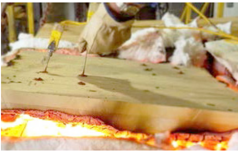
Mercer CLT - Char Rate Testing
