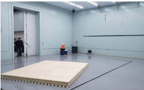
Mercer CLT - Acoustic NRC Testing
