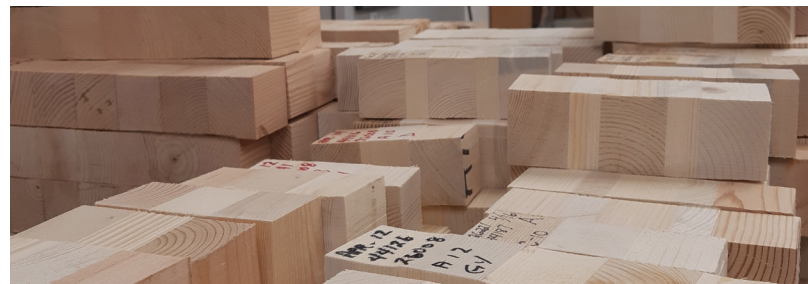
Figure 6: Glue-bond sample test blocks
